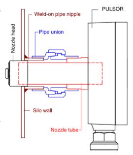
Three different Pulsor types are available, which differ in air consumption and effective range. Number, type and arrangement of the Pulsors on the silo, as well as the optimum activation cycle, depend on the flow characteristics of the bulk solid, the silo shape and the procedural requirements.
