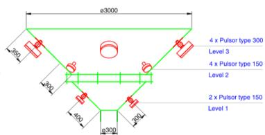
... here, too, one no longer has to knock with a hammer. The bulk material is fluidized by the injected air and flows out...
