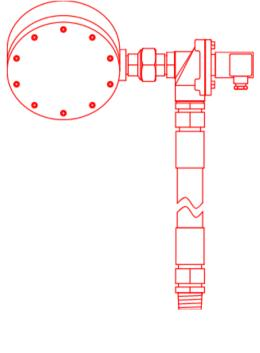
In general, the pulsors should be activated for only approx. 0.8 s each time. The pause time until the next activation is between a few seconds and a few minutes,
